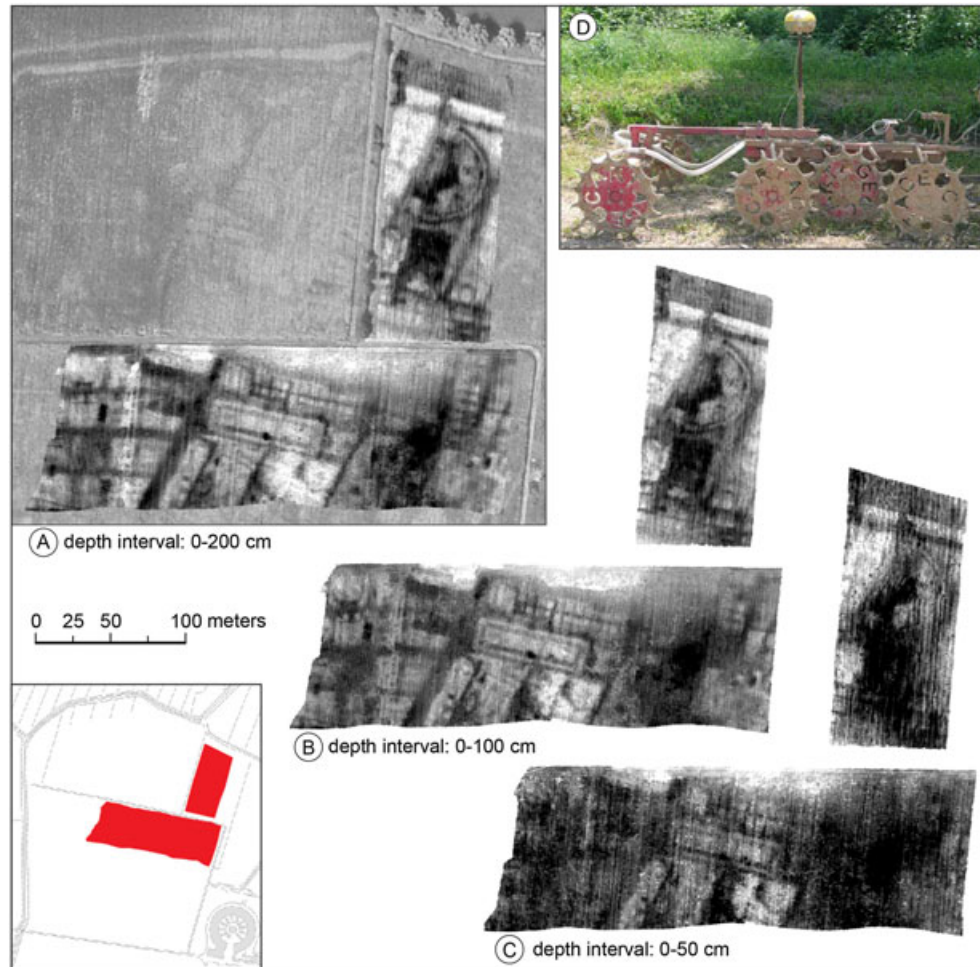
Figure 5. Map of the apparent resistivity obtained through automatic resistivity profiling (ARP©) considering different pseudo-depth intervals: (A) 0–200 cm; (B) 0–100 cm; (C) 0–50 cm. (D) Picture of the device (Dabas, 2009). Image in the background is a grey-tone version of Figure 2B. This figure is available in colour online at wileyonlinelibrary.com/journal/arp
